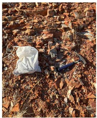
Plate 3.1 Example of Rock Chip Sampling of Outcrops, and Rock Hammer typically used
