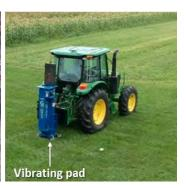
Plate 3.4 Examples of Energy Source Vehicles with Vibrating Pad (EnviroVibe, Bobcat, Tractor)
