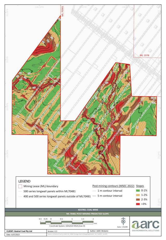
Figure 9: Inferred slope gradient classes post-mining (MSEC [2022] predicted subsidence DEM)
