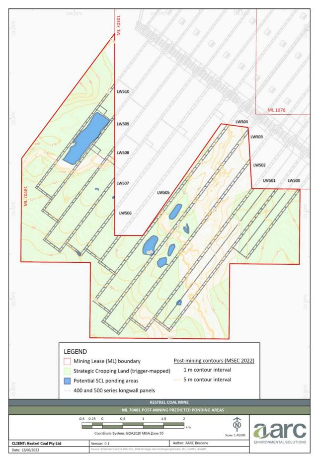
*Figure 11:* Inferred ponding subsequent to subsidence (revised mine plan incl. LW510)
