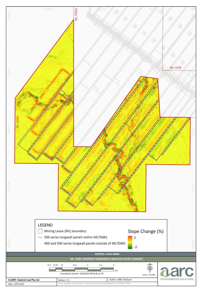
*Figure 10:* Inferred subsidence-induced slope changes between +2% and -2%
