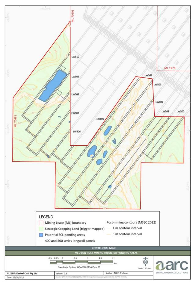
*Figure 9:* Inferred ponding subsequent to subsidence (revised mine plan incl. LW510)
