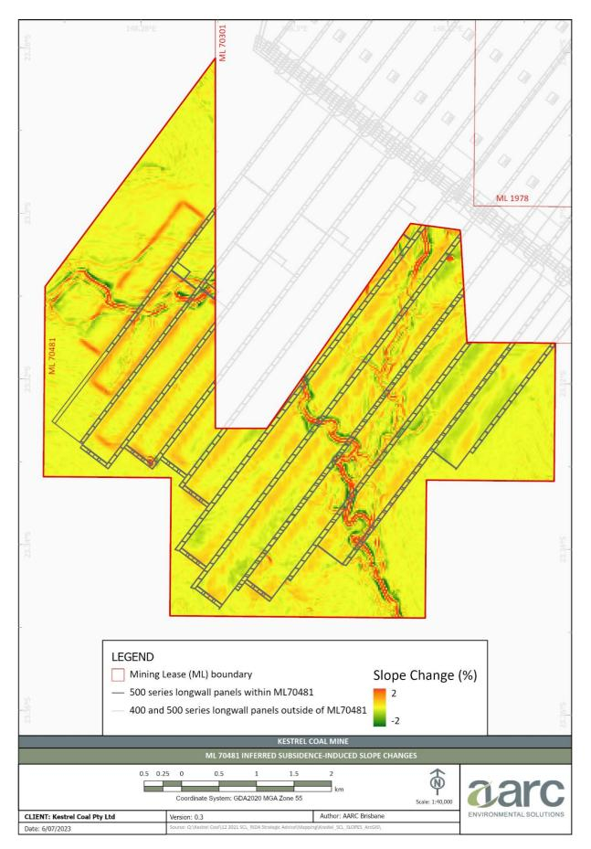
*Figure 8:* Inferred subsidence-induced slope changes between +2% and -2%
