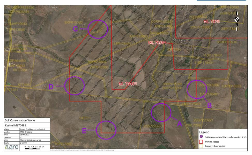
*Figure 6: Soil erosion structures on ML70481*
